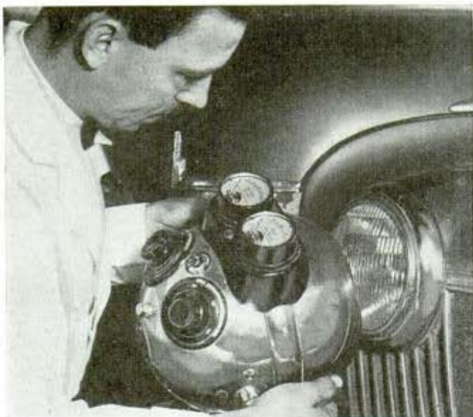
Top, headlight-testing "bomb" fits against headlight to measure its output of light. Below, bathe the air filter in gasoline every few thousand miles, then dip it in light oil
